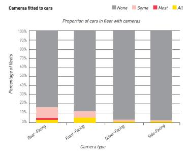
Few car fleets surveyed have cameras fitted. Reversing cameras are the most common, and are present on vehicles in 18 fleets (16%); front-facing cameras in 13 (12%), side-facing in three (3%), and driver-facing in three (3%).
