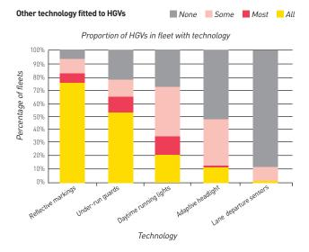
Under-run protection is required by EU law for trucks over 3.5 tonnes. In our survey responses, it is present on all HGVs in 80% of fleets. Reflective markings were also common, being on all vehicles in 92% of fleets.
