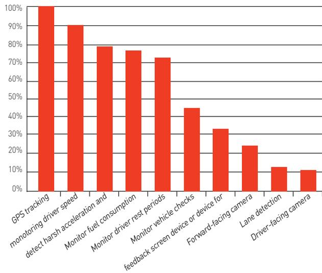
GPS tracking, speed monitoring and detecting harsh acceleration and braking are all common features of telematics systems, whereas forward and driver-facing cameras, and lane detection, are rare. Two fleets noted that they were updating their telematics system to more advanced driver-monitoring systems, and another noted that their telematics system had additional features that they were not making use of.
