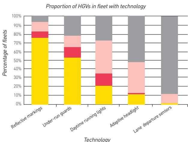
Under-run protection is required by EU law for trucks over 3.5 tonnes. In our survey responses, it is present on all HGVs in 80% of fleets. Reflective markings were also common, being on all vehicles in 92% of fleets.
