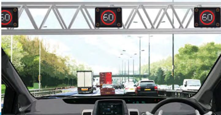
Controlled motorways have three or more lanes with variable speed limits. The hard shoulder is separated from live lanes by a solid white line and should only be used in a genuine emergency.
