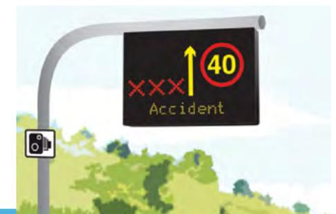
We use a red X symbol to show that a lane is closed because of an incident or people working on the road. Driving in a lane with a red X symbol is dangerous and drivers must **not** use it.
